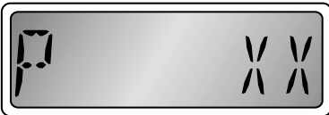
Port Sensor - Starboard blocked
