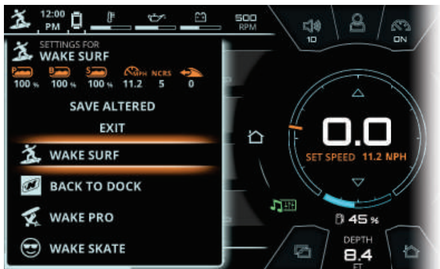
FIG. L - DROP-DOWN MENU AFTER PRESSING THE USER BUTTON ON HELM COMMAND
