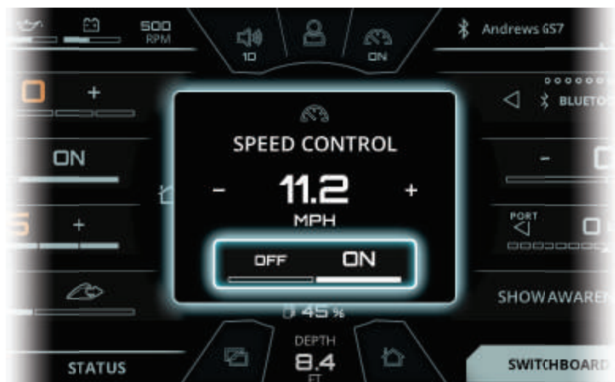
FIG. M - POP-UP AFTER PRESSING THE SPEED CONTROL BUTTON ON HELM COMMAND
