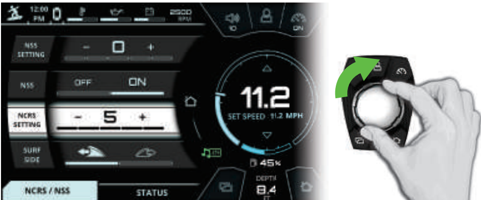
FIG. I - ROTATING CLOCKWISE TO INCREASE A SETTING
