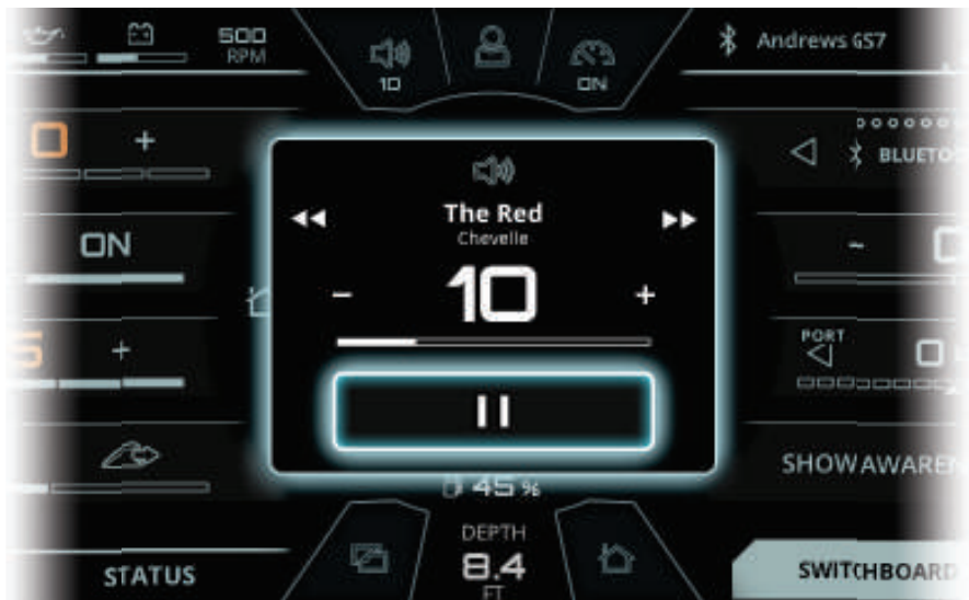
FIG. K - POP-UP AFTER PRESSING THE VOLUME BUTTON ON HELM COMMAND
