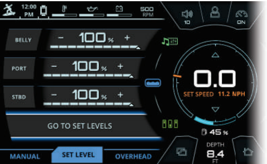
FIG. BB - SET LEVEL TAB ON THE BALLAST MENU
