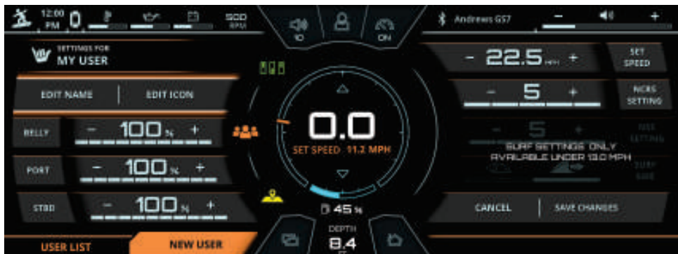
FIG. JJ - NEW USER TAB (EDIT USER SCREEN TO ADJUST SETTINGS)
