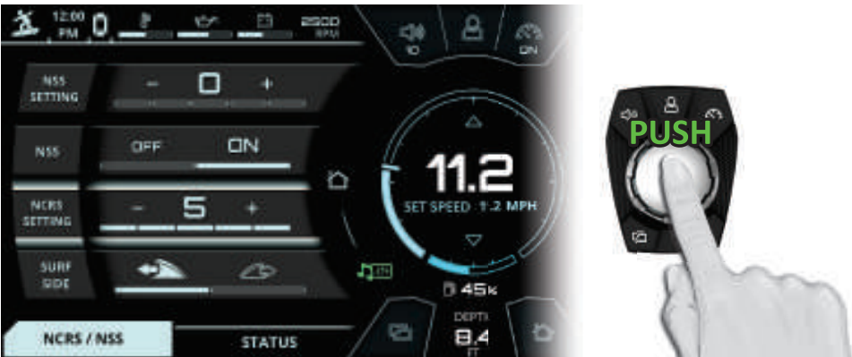
FIG. J - PUSHING DOWN TO DE-SELECT A SETTING (THE NCRS SETTING IN THIS EXAMPLE)
