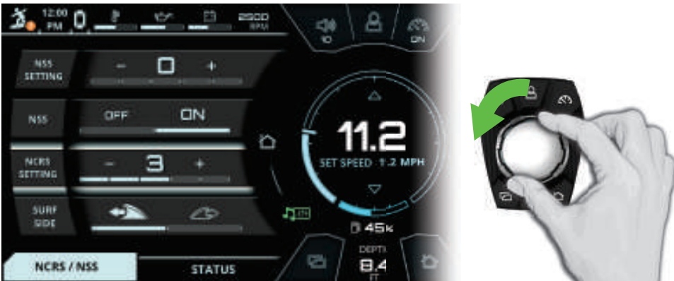
FIG. G - ROTATING COUNTER-CLOCKWISE TO HIGHLIGHT A DIFFERENT SETTING
