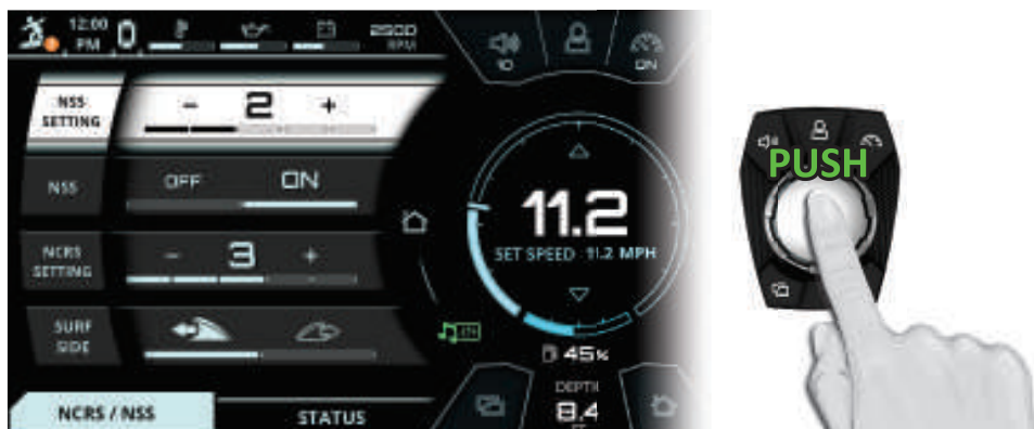
FIG. D - PUSHING DOWN TO SELECT A SETTING (THE NSS SETTING IN THIS EXAMPLE)
