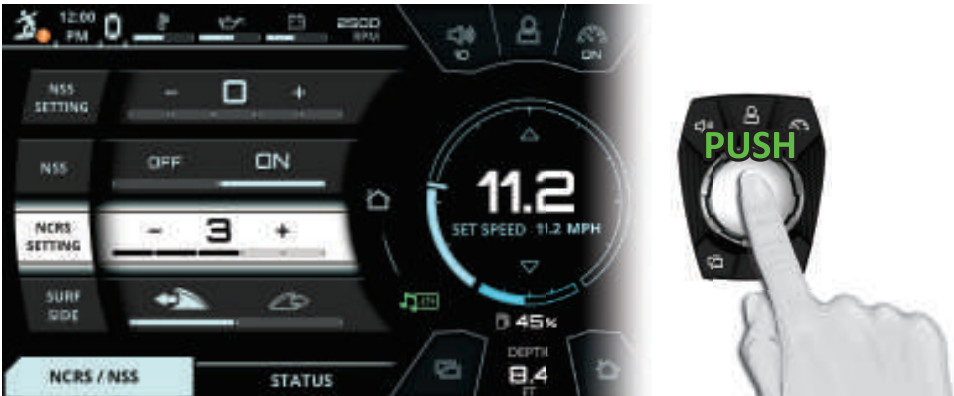
FIG. H - PUSHING DOWN TO SELECT A SETTING (THE NCRS SETTING IN THIS EXAMPLE)
