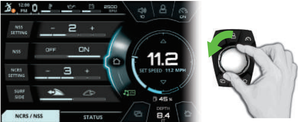
FIG. B - ROTATING COUNTER-CLOCKWISE BACK TO THE HOME MENU FROM THE MEDIA MENU
