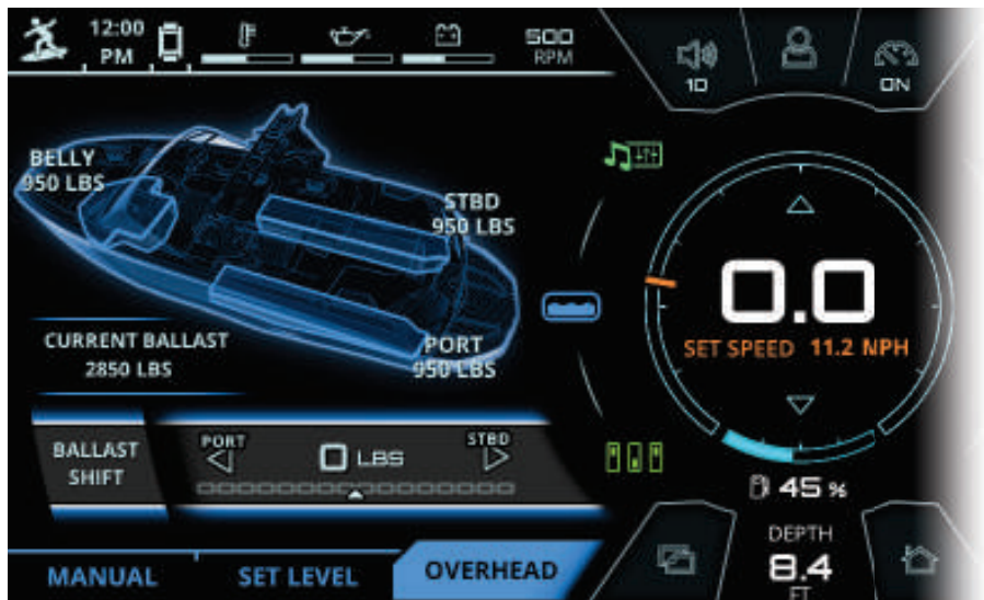
FIG. CC - OVERHEAD TAB ON THE BALLAST MENU
