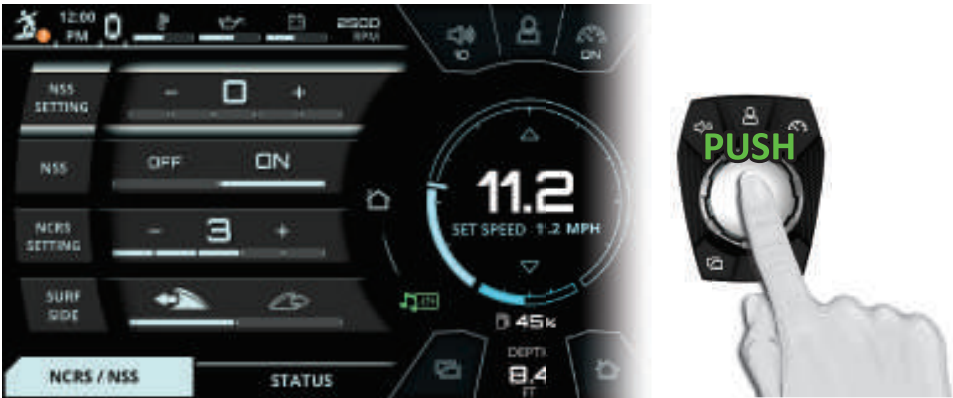
FIG. F - PUSHING DOWN TO DE-SELECT A SETTING (THE NSS SETTING IN THIS EXAMPLE)
