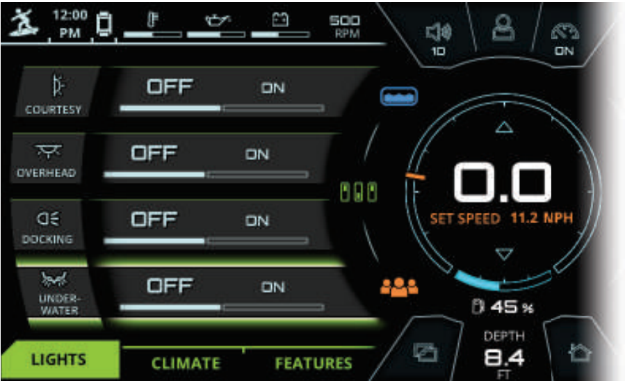
FIG. DD - LIGHTS TAB* ON THE SWITCHING MENU
