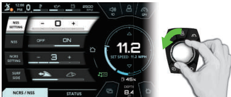
FIG. E - ROTATING COUNTER-CLOCKWISE TO DECREASE A SETTING
