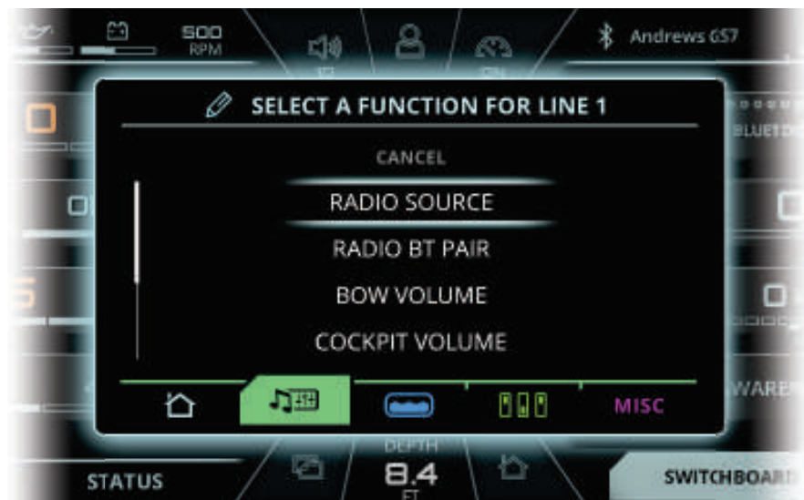
FIG. WW- SWITCHBOARD TAB ON THE RIGHT SECTION OF THE DISPLAY
