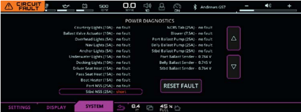
FIG. N4 - POWER DIAGNOSTICS ON PREFERENCES MENU
