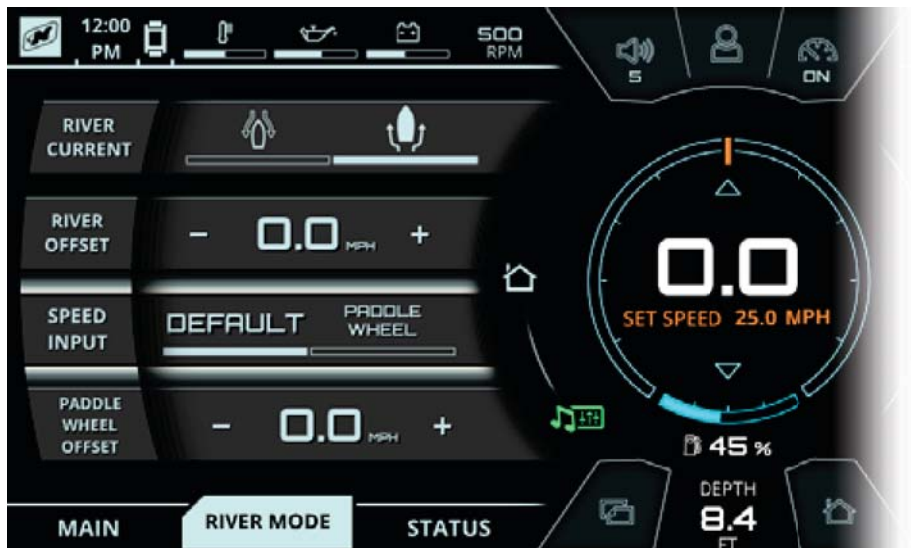
FIG. E2 - RIVER MODE FOR BOATS EQUIPPED W/ PADDLE WHEEL
