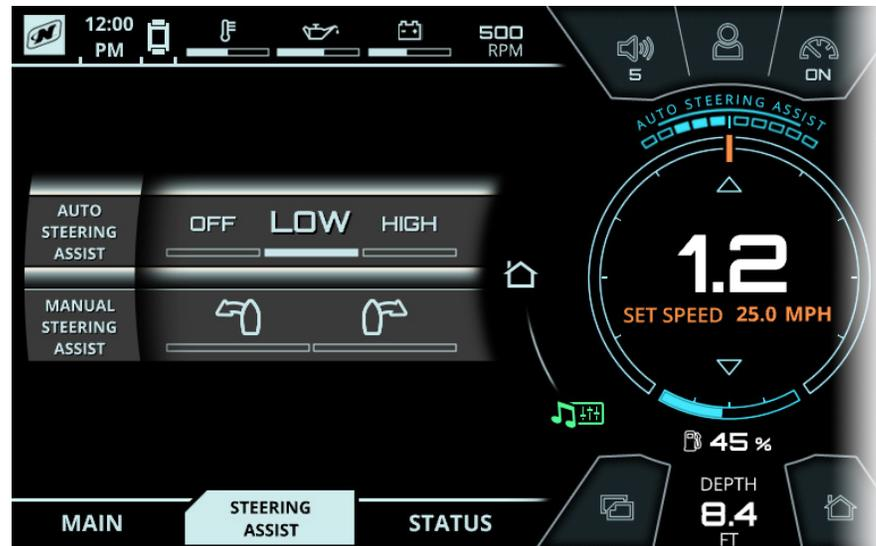
FIG. F2 - AUTO STEERING ASSIST SET TO LOW AND THRUSTER IN USE (BLUE GRAPHICS)
