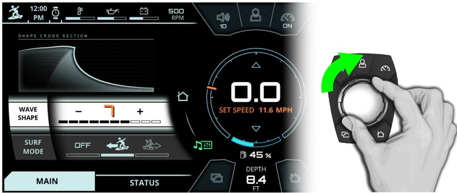
FIG. A5 - ROTATING CLOCKWISE TO INCREASE A SETTING
