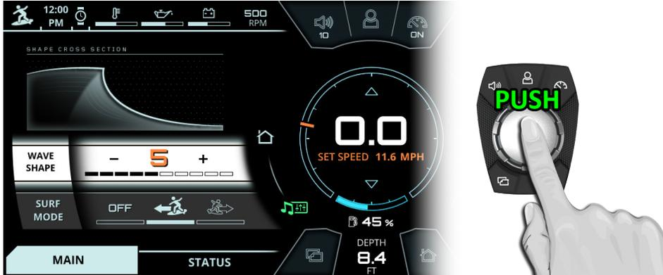
FIG. A4 - PUSHING DOWN TO SELECT A SETTING (THE WAVE SHAPE SETTING IN THIS EXAMPLE)
