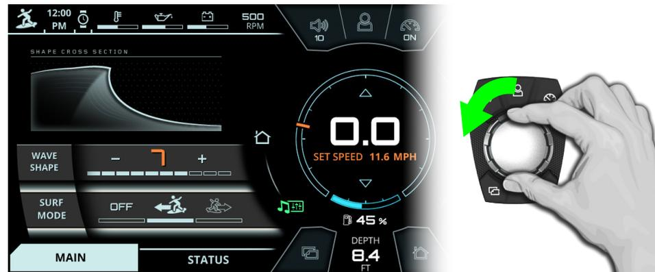
FIG. A7 - ROTATING COUNTER-CLOCKWISE TO HIGHLIGHT A DIFFERENT SETTING
