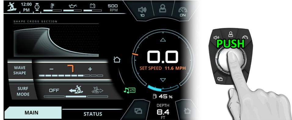
FIG. A6 - PUSHING DOWN TO DE-SELECT A SETTING (THE WAVE SHAPE SETTING IN THIS EXAMPLE)
