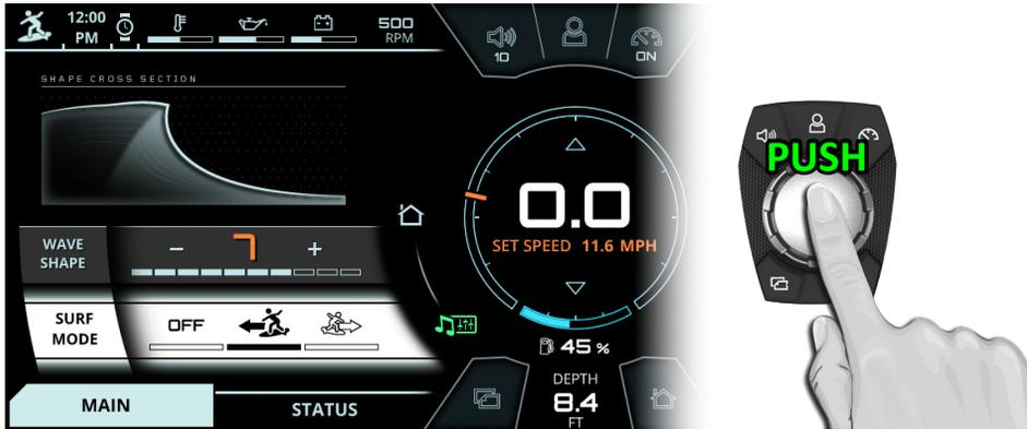
FIG. A8 - PUSHING DOWN TO SELECT A SETTING (SURF MODE SETTING IN THIS EXAMPLE)
