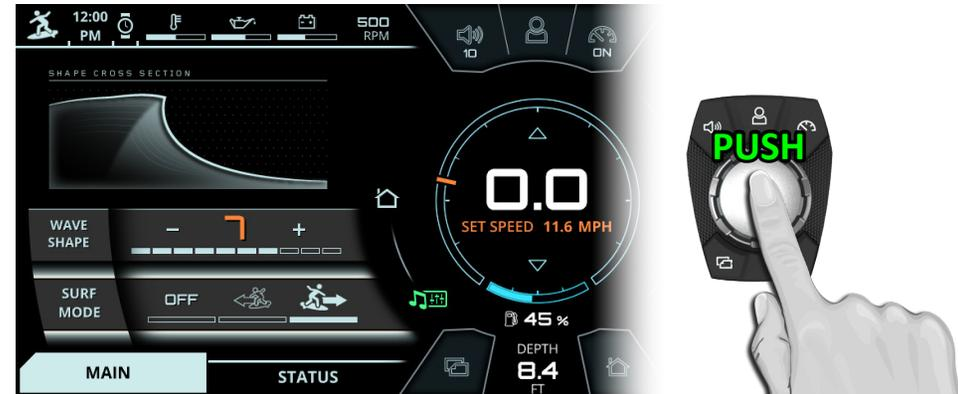
FIG. A10 - PUSHING DOWN TO DE-SELECT A SETTING (THE SURF MODE SETTING IN THIS EXAMPLE)
