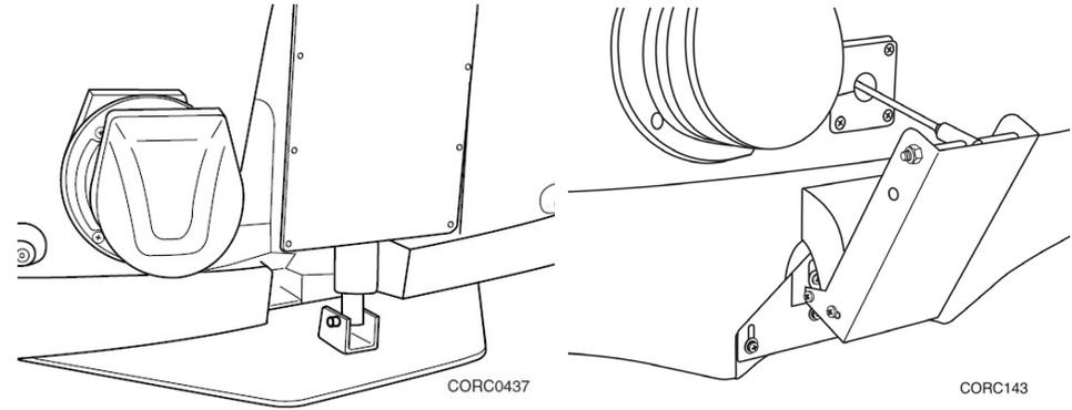
FIG. C4 - NAUTIQUE HYDRO-PLATE, LOCATED AT THE REAR OF THE BOAT (G and GS Series Boats)
