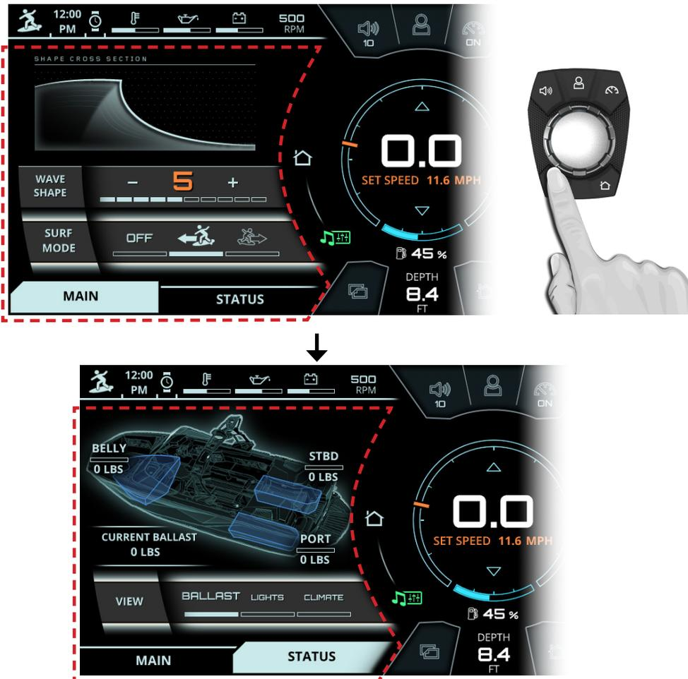
FIG. B6 - PRESSING THE TAB BUTTON ON HELM COMMAND TO CHANGE TO THE "STATUS" TAB
