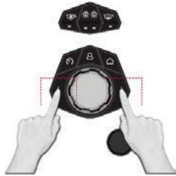
Activate Helm Command into Fail Safe Mode
