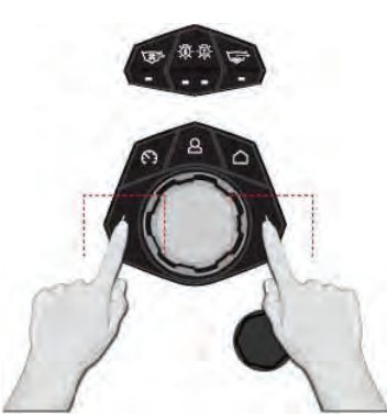
Activate Helm Command into Fail Safe Mode
