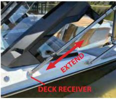
Unzip and remove the bimini cover boot. Adjust the forward support poles to the fully extended position and engage them into the forward deck receivers (*Figure 9*).
