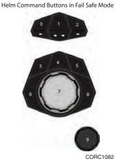
The Helm Command buttons will automatically exit the Fail Safe Mode when it sees a valid User Code has been entered or when the battery switch is turned off.
