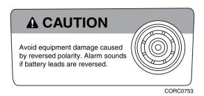
**NOTE:** When connecting the battery terminals to the battery, always connect the RED terminal to the positive (+) battery post first. Then connect the black terminal to the negative (-) battery post.
