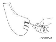
If the boat is pulling port **(A)**, rotate the foil to port **(B)** and tighten screws. If the boat is pulling starboard **(C)**, rotate the foil to starboard **(D)** and tighten screws. Always remember that movement of the trailing edge of the foil to one side will cause the steering to pull to the opposite side.
