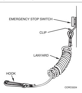
To attach a lanyard, connect the clip to the emergency stop switch and the hook to a strong piece of clothing on the operator, such as a belt loop.
