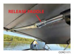
Press the paddle on the center of the tension rod to release it. Use the black clip to secure the center tension rod to the frame. Fold the bimini and lay it back *(Figure 13)*.
