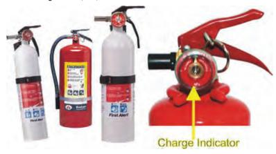
5-B extinguishers are required for boats less than 26 feet in length. Check periodically to ensure that the extinguisher is in working condition and fully charged. Disposable (non-rechargeable) fire extinguishers with a date of manufacture stamped on the bottle older than 12 years must be removed from service and no longer count towards the minimum carriage requirements. Check local, state and federal agencies as to laws and regulations.
