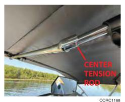
Rotate the bimini to the fully up position. Push up on the center tension rod until it clocks. It will lock into position *(Figure 10)*.
