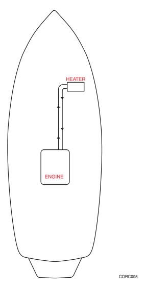
The heater system has a heating core, ducts, diffusers and a high-speed fan to deliver heat to the cockpit and windshield. The duct diffuser at the windshield can be closed and rotated to direct air flow. The floor ducts can also be closed to control air flow. The aft duct and diffuser can be pulled out of its socket to direct flow in other locations of the cockpit. The heating unit is located under the driver's dash pod.
