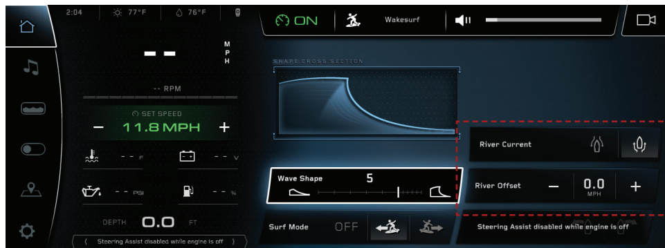
GPS RIVER MODE FOR BOATS EQUIPPED WITHOUT PADDLE WHEEL
