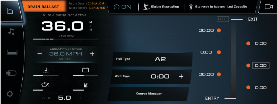
DRAIN BALLAST BUTTON/GRAPHIC (TANKS SHOULD BE EMPTY FOR SLALOM/JUMP EVENTS)
