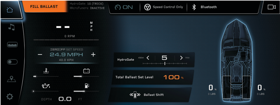
FILL BALLAST BUTTON/GRAPHIC (TANKS AREN'T CURRENTLY AT THE 100% SET LEVEL)
