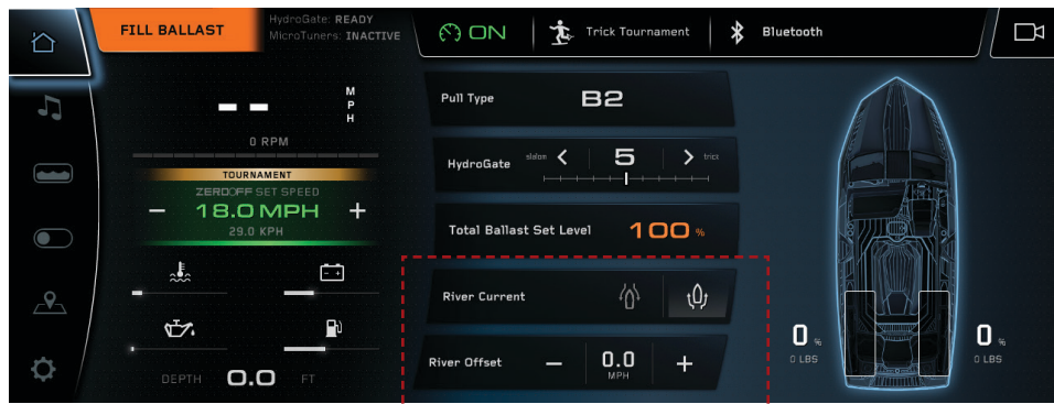
GPS RIVER MODE FOR BOATS EQUIPPED WITHOUT PADDLE WHEEL
